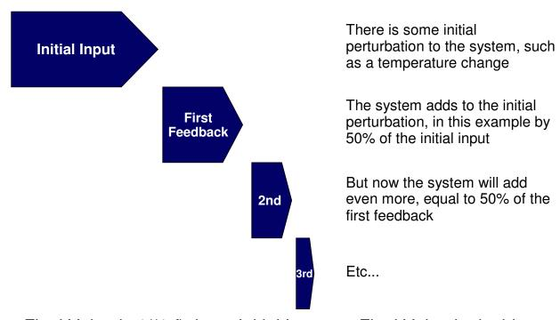
Final Value is 1/(1-f) times Initial Input, so Final Value is double the Initial Input when f=50%
